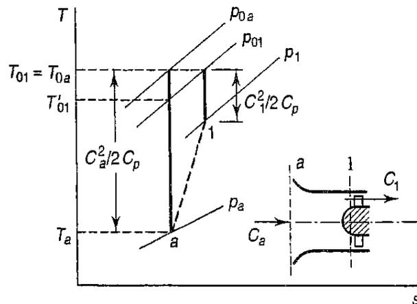
The main function of intake is to minimize the pressure loss upto the compressor phase while ensuring that the flow enters the compressor with uniform pressure and velocity.
